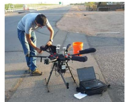
Testing the new drone-mounted LiDAR system
